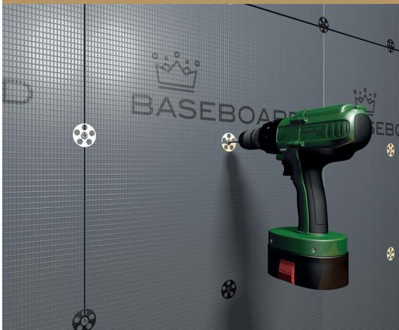
6. When all the panels are securely fixed to the studwork ensure to waterproof all joints with Baseboard Waterproof Tape (for wet zones - tape a minimum of 300mm past the wet zone area). Ensure all joints and screw heads are taped. If preferred, Baseboard AquaTank Fleece+ and Neo-Flex can be used for all board-to-board joints.
