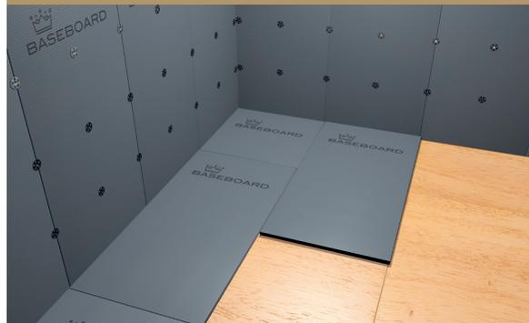
3. When the adhesive is applied, place the Baseboard Panels directly onto adhesive layer.
