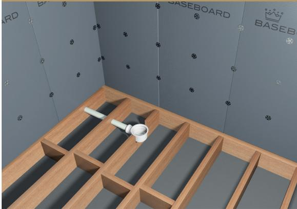
4. All plywood infill pieces must be fixed to the battens. **Pro Tip** – Mark the location of pipes and wires on joists before fixing plywood inlays.
