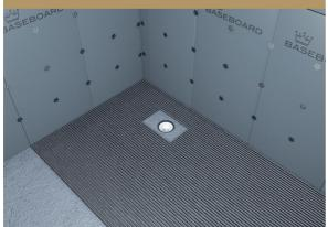
3. Carefully place the Baseboard Shower-Tray directly onto the adhesive layer, ensuring the alignment of the outlet in the tray with the trap. Tamp the tray down so it makes full contact with the adhesive.
