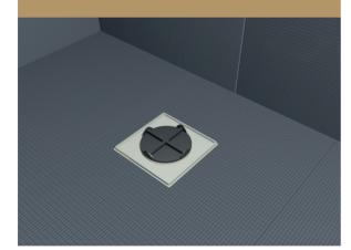
6. Continue fitting Baseboard Panels to the remainder of the floor, ensuring all the boards are tamped down and level. Once adhesive is dry, insert bucket and dip tube. Ensure to waterproof all joints with Baseboard Waterproof Tape (for wet zones - tape a minimum of 300mm past the wet zone area). Ensure all joints and screw heads are taped. If preferred, Baseboard AquaTank Fleece+ and Neo-Flex can be used for all board-to-board joints.
