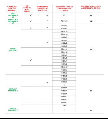
s1: low smoke emission s2: medium smoke emission s3: high smoke emission
