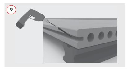
— Predrill a hole like the pic shown above and then screw the decking boards to the joist.
