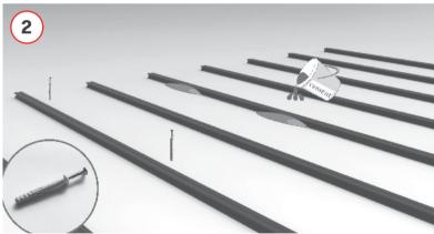
— Fix the joists tight onto the ground by using screws or cement.
