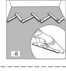
11. Dismantle and cut Number the panels from  ${\bf 1}$  to  $\ldots$  . This will allow you to keep the panels in order. Dismantle the panels and cut them to size along the previous marked line.
