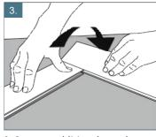
3. Connect additional panels Next panel is an A-panel. Again, press the long side of the new A-panel at an angle against the short side of the previous B-panel and fold down. Continue like this with as many panels as may fit along the starting wall.
