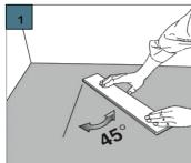
1. Getting started. Choose a wall to start at and begin installing at the left corner. Start with an A-panel and place it with its long side  $marking \, facing \, the \, left \, wall \, at$ an angle of 45°. Make sure that the distance between the left wall and the panel is less than the length of one panel.
