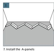
Continue from the left to the right and install all the A-panels in the second row. Finish with a piece of panel cut tosize (step 5).
