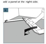
6. Start the second row Start the next row with an A-panel. Place the new panel against the previous row and fold down.
