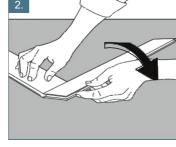
2. Connect next panel Continue with a B-panel. Press the long side of the B-Panel at an angle against the short side of the previous installed Apanel. Fold down the B-panel flat to the floor to lock the panels tightly together. Check that the grooves on the two panels form a continuous line.
