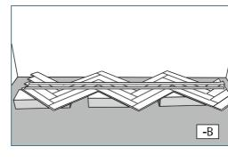
Leave the left end-panels uninstalled. Tape along the marked line and place the flooring on top of a few flooring packages. Cut along the marked line. Then put the adjusted rows into place. Complete the first rows by installing the remaining end-panels. Start with the end-panel in the last row and finish at the first row
