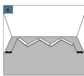
4. Center the first row Check that the first row of panels is centered along the starting wall. Make sure that the distance to the walls on both sides are less than the length of one panel. If not,
