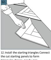
triangular shapes, one by one. Start installing the triangles from the left corner. It is recommended to use glue to fix the smallest parts of the triangles into place by applying a small quantity of glue inside the groove.
