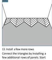
each row from the left to the right with the A-panels, finish with the cut piece of panel (step 5) and then install all the B-panels in the row. Finish with the left end panel, cut to size.
