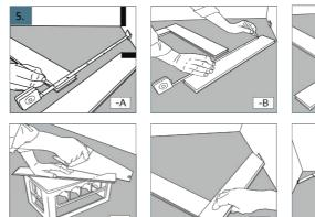
5. Cut the end panels to size Measure and cut the end panels to size using a fine toothed saw. Finish the first row with the cut end panels. Make sure that you leave a gap of 10mm to each wall.
